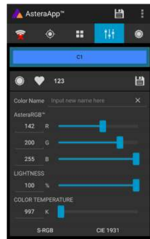
The editor will open. RGB values can be adjusted directly. Also a color temperature can be converted to RGB.
